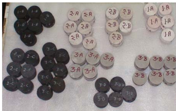
Figure 9: Rock samples prepared for SHPB test.
