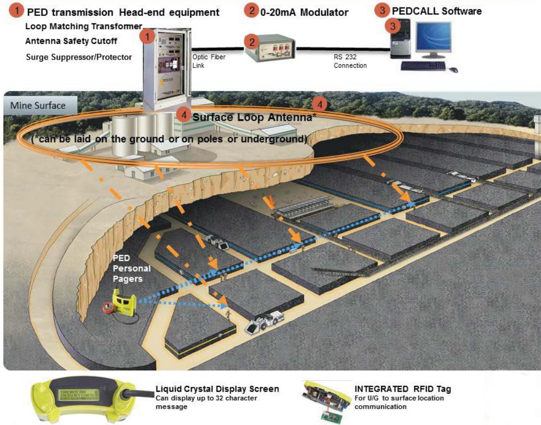
Figure 5: Through The Earth Ultra Low Frequency Emergency Messaging System
