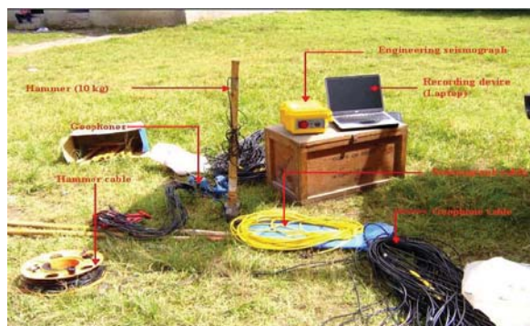
Figure 3: Various components of the MASW system
