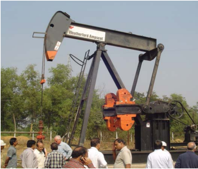
Fig 3: Dewatering and recovery of gas in CBM well by SRP pump at Moonidih
