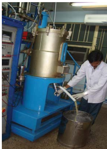
Mass production of biopesticide in a Fermentor (100 l)
