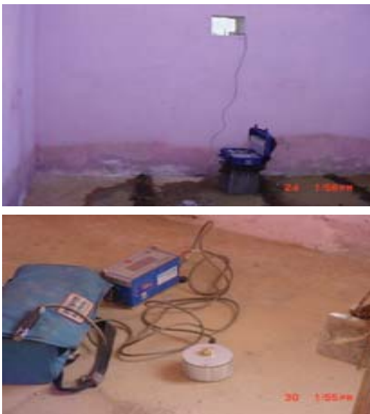
Photograph 4: Monitoring of response of the brick-mud structure with cement plaster to blast induced vibration at Kumdanda Project.
