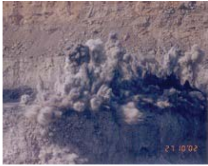
Photograph 2: Rock movement and venting of gases in top initiation at Ksumunda project.
